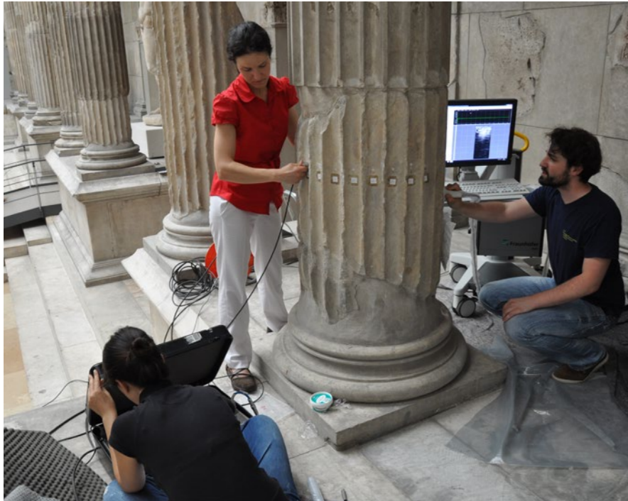
Figure 18: Ultrasound Tomography System: classical method with two probes (left), new approach using many elements along a belt (right) © Peter Weber, Fraunhofer IBMT
