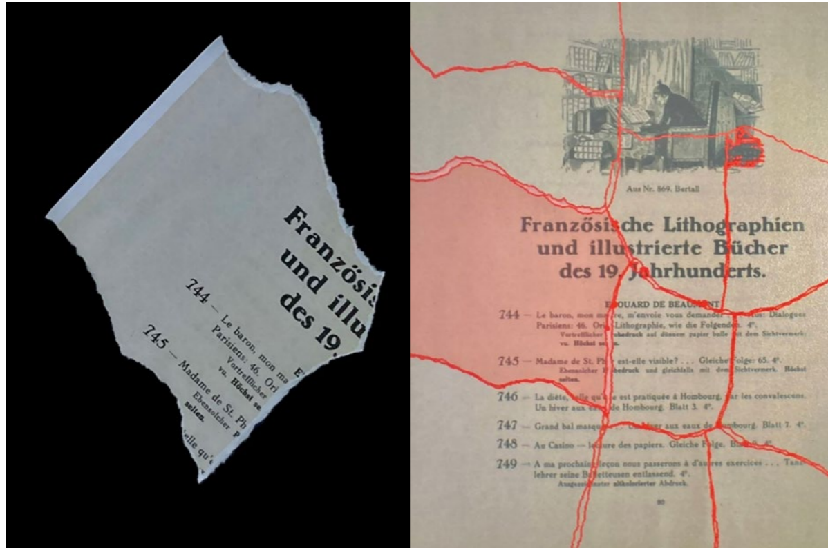
Figure 25: An exemplary fragment placed loosely under a camera (left) and the projection based on it on a white background with the target pose of the fragment highlighted in red (right) © Fraunhofer IPK
