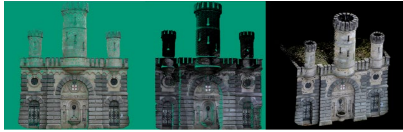
Figure 5: Photogrammetric (left) and scanner data (center) were combined into a highly detailed 3D point cloud of the Wasserschlosschen (right). © Fraunhofer IPM
