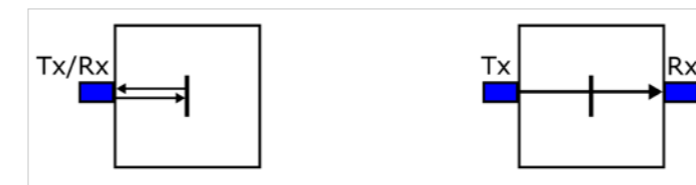
Figure 16: Pulse echo and transmission mode © Peter Weber, Fraunhofer IBMT
