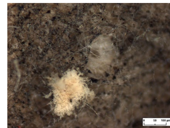
Figure 20: Light micrograph, magnification 155x, fungal hyphae and fungal spores on the paper surface © Fraunhofer FEP
